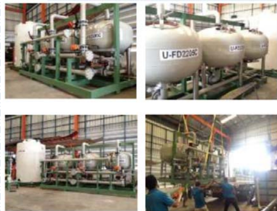
Automatic Sand Filter 3 Units.
